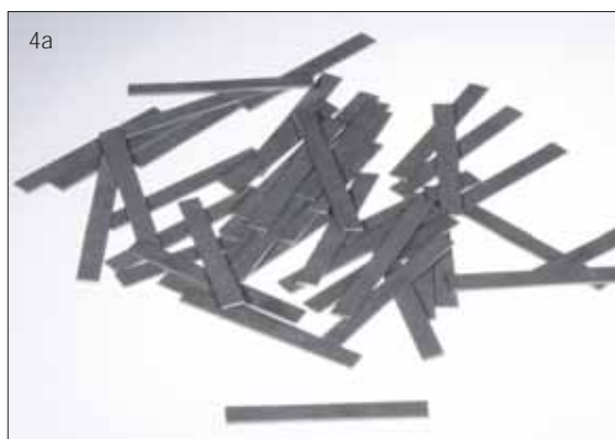
Fig. 4a Fabrication of the Schwickerath test pieces according to EN ISO 9693:2000
