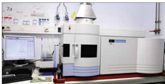
Fig. 7a and 7b ICP spectrometer used for analysis of the metal ions released into the solution and determination of the loss of mass
