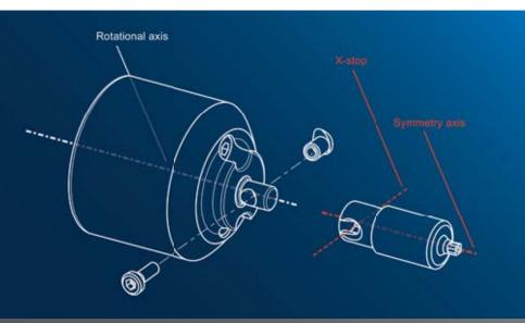
**07** Schematic representation of the relevant coordinates and parameters for positioning the Preform blank on the blank holder. The symmetry axis of the blank must be aligned exactly to the rotational axis of the holder. Two precise countersunk screws ensure the central alignment on the rotational axis; the implant connection geometry remains untouched
