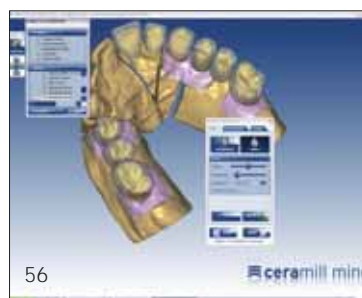
Fig. 54 to 56 The virtual design corresponds exactly to the wax-up in shape, function and aesthetics. With a click of the mouse the digital design can now be "shrunk" to the framework that supports the porcelain veneer
