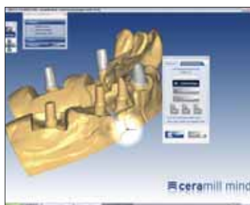
Fig. 49 and 50 The stripe-light scanner has captured all relevant areas. The software defines the preparation margins automatically with the click of the mouse. The recommendation can be checked and, if necessary, adjusted manually
