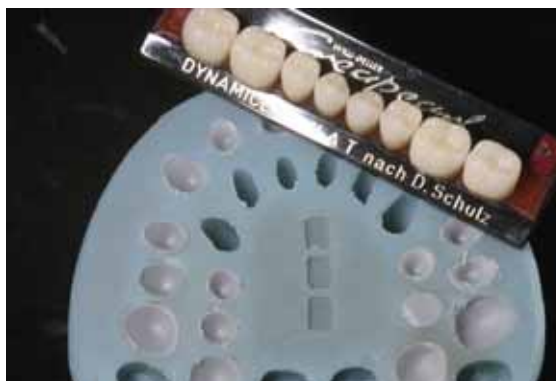
Fig. 7 An appropriate set of denture teeth was duplicated using 9:1 silicone to ensure a consistent, efficient procedure. The moulds could be filled with wax, ...
