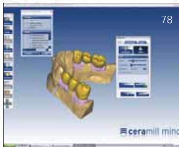
Fig. 80 Two laser-sintered CrCo bridge frameworks were manufactured in a milling centre. At the same time we utilised the shell of the situation scan to generate a fully anatomical PMMA temporary restoration
