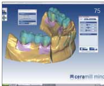
Fig. 75 to 79 A situation scan, gingiva scan and model scan are also completed in the lower jaw based on the wax prototype and the bridges were designed as already described
