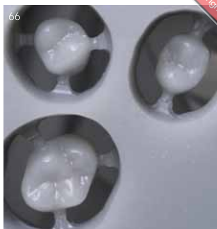
Fig. 64 The correct size of blank (here zirconia) was inserted in the milling unit
