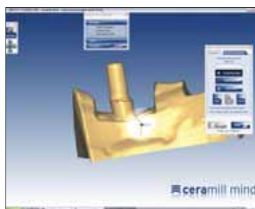
Fig. 49 and 50 The stripe-light scanner has captured all relevant areas. The software defines the preparation margins automatically with the click of the mouse. The recommendation can be checked and, if necessary, adjusted manually
