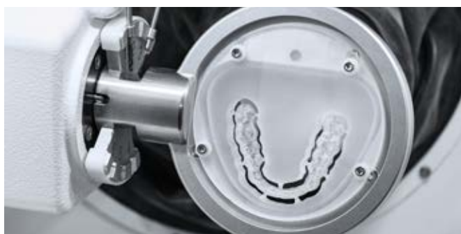
Easy, reproducible splint fabrication using Ceramill CAD/CAM
