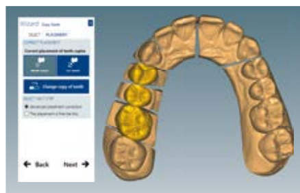
Copy or mirror teeth to produce a uniform tooth shape/structure in a jaw
