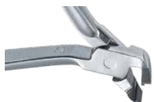
Distal end cutter sterilizable For shortening the archwire ends in the multi-bracket technique. Wire holder. Inserts made of hard metal. Max. wire thickness: \square 0.56 x 0.70 mm / 22 x 28
