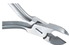
Side cutter Medium sterilizable For cutting wires and arches. Inserts made of hard metal. We do not recommend using the front third of the cutters for cutting wires with the maximum indicated thickness! Max. wire thickness: \varnothing 0.7 mm, hard
