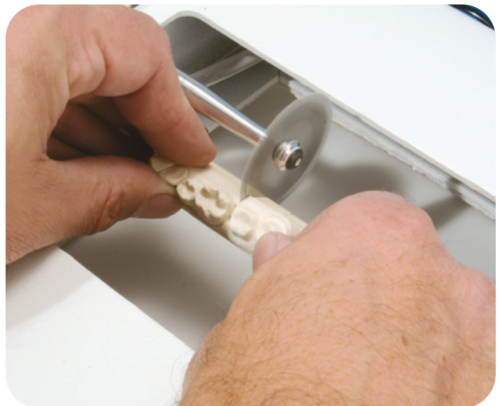
The blue table top can be flipped up to use the diamond disk lathe style for making buccal and lingual cuts or can be top cut with a hand saw to complete the die section.
