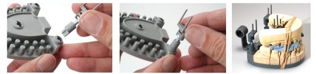
9. Photo right; The Flex Arm Hinge for the opposing side is inserted through the opening of the V2 silicone Pic-Up Cup. Also shown is the OPTIONAL Split Cast Plate (see Split Cast Plate) which can be retained into the cast for magnetic attachment to semi or fully adjustable articulators.
