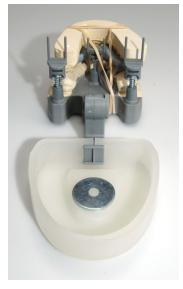
After the plaster has set up, remove the cup, rubber bands and break away the retainer tabs (left photo) from the Stop Heads to allow the articulator to open up.
